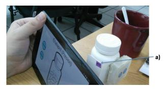
Figure 4. Remind-Me is moved close to GUIDe-Me when the medication has been taken to record it and to deactivate the dose light.
