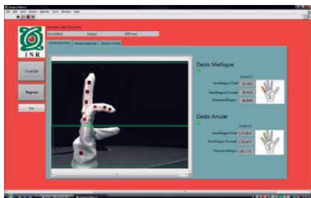
Figure 4. Measurements of the ring and little finger of the mechanical mannequin.
