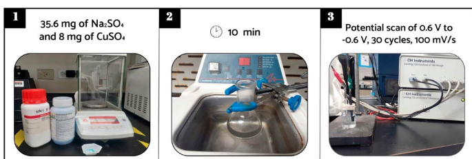
FIGURE 5. Electrodeposition of Cu on MWCNT-Nf.
