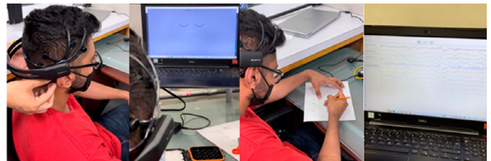
FIGURE 9. EEG acquisition process with the Epoc+ BCI.
